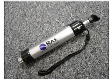
The tubes are available in different ranges 1-30 ppm, 5-100 ppm, and 25 - 500 ppm. The lower range offers very precise measurement in low ammonia situations. The 5-100 ppm range tubes allow for a wider range of ammonia conditions and can be used to determine ammonia concentration to approximately 5 ppm level.
