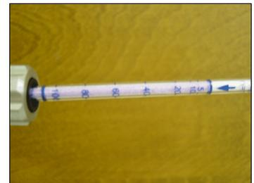
The accuracy of gas detection tubes can vary significantly (+/- 10 to 20%) because of the difficulty involved with determining exactly where along the length of the tube the color changes from purple to beige, sampling procedure errors, as well as environmental factors. If a highly accurate reading is desired multiple samples should be taken.
